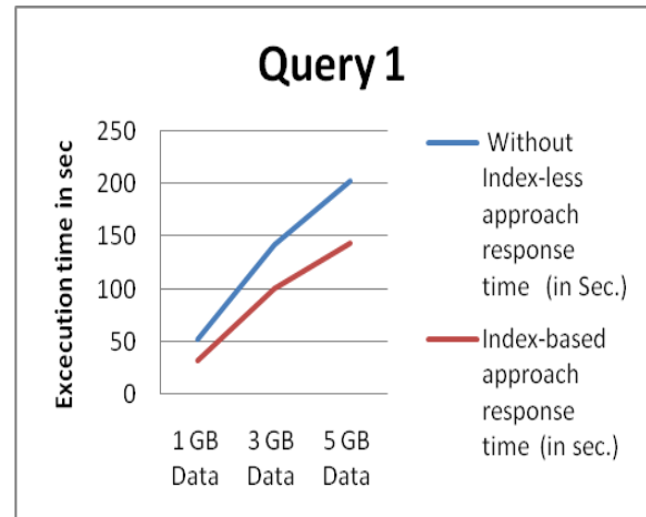
Figure 3: Query1 response time without index based / with index-based approach on single node setup
