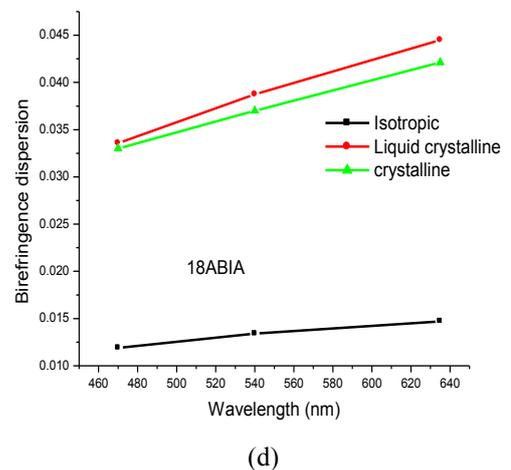
Figure 4. Birefringence of (a) 8ABBA; (b) 18ABIA; birefringence dispersion of (c) 8ABBA; (d) 18ABIA
