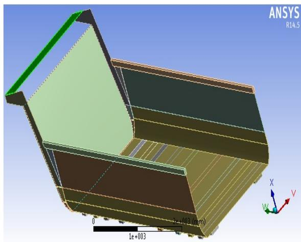
Figure 2: Pro-E model of Hardox 400 Tipper body
