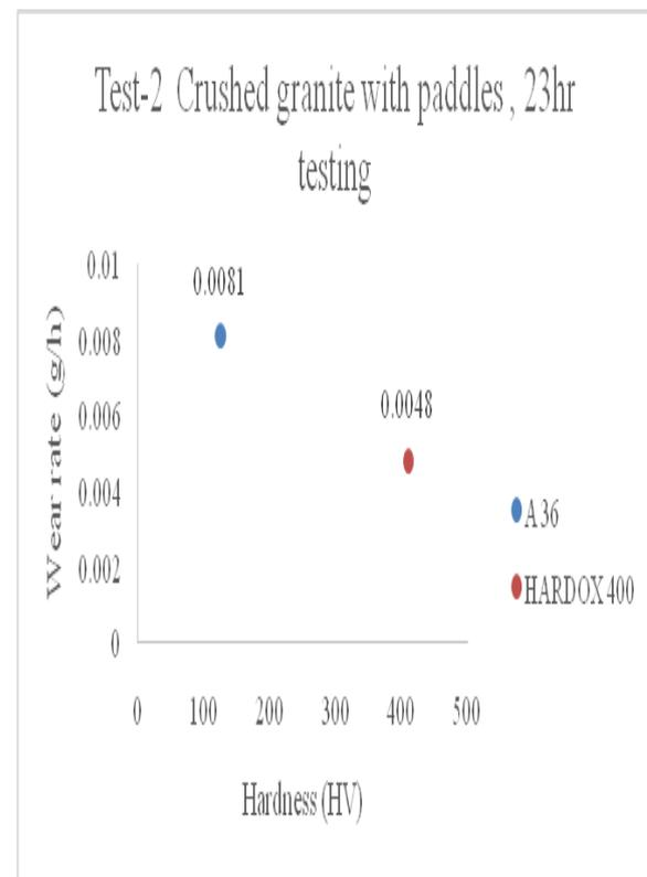
Figure 6: Test-2 Crushed granite with paddles, 23hr testing
