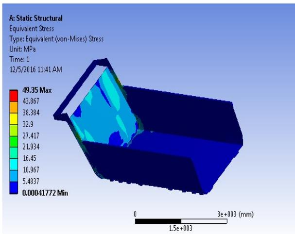
Figure 5: Head Stress Developed in HARDOX 400 Tipper Body
