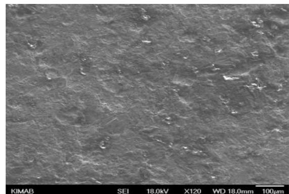
Figure 10: HARDOX 400 shows less deformed surface
