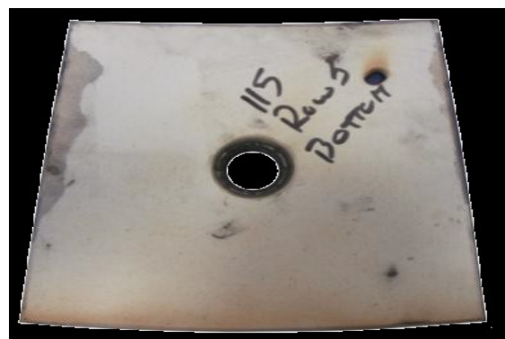
Figure 3: Component subjected to thermal paint
