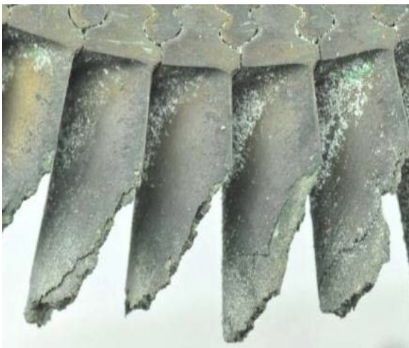
Figure 1: Creep Failure of Turbine Blade
