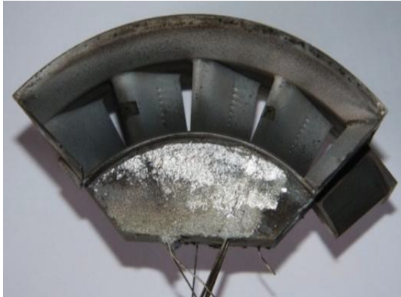
Figure 2: Point of Application of thermal paint
