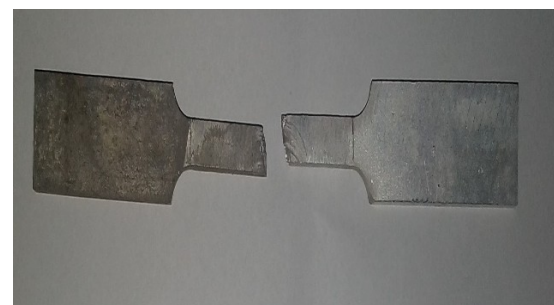
Figure 3. Tested Weld Joint
